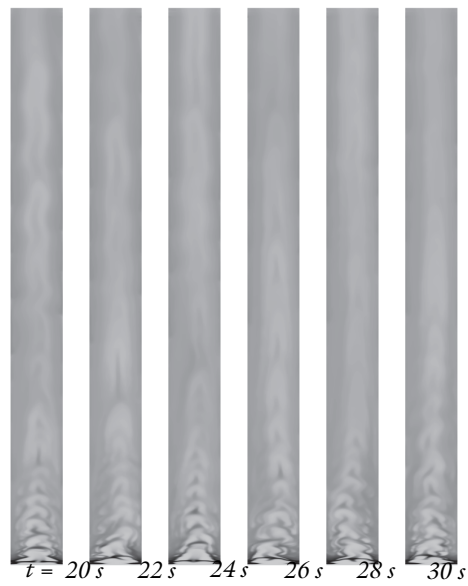
Figure 5: Snapshots of the dispersed phase volume fraction during the steady-state operation. Black indicates high volume fraction. The bed width has been scaled by a factor of ten.
