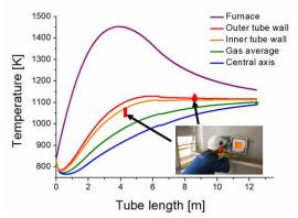
Figure 3. Temperature distribution along the furnace and the catalytic tube. Lines: simulation. Symbols: experimental data.
