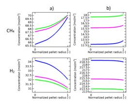
Figure 5. Simulated concentration profiles of CH<sub>4</sub> and H<sub>2</sub> in catalyst pellets at different positions along the tube: a) z=0.6 m (minimum temperature); b) z=12.43 m (outlet). Radial position: tube axis (green line), middle of radius (magenta line), and inner tube wall (blue line).
