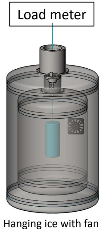
Initial model predictions assuming only radiative heat transfer through MLI gave a good idea of expected thermal performance for early prototype Dewars.
