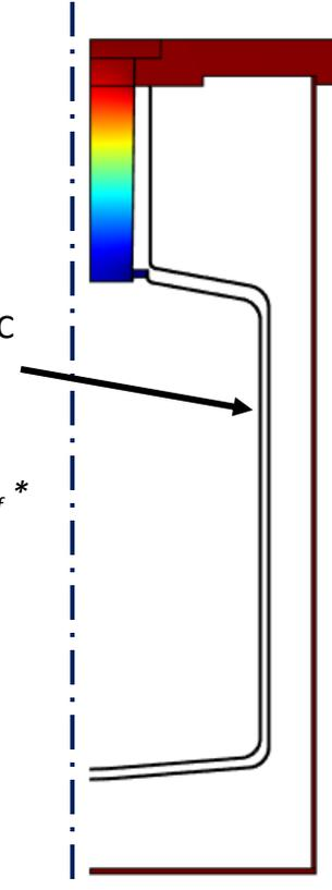
Instead of adding a complex conduction fitting equation to the COMSOL model, experimental data could be used to tune  $\epsilon_n$  to compensate for lower effective emissivities between the MLI layers. ***The resulting model fit experimental data well over a range of MLI layers.***
