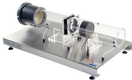
Figure 1. FM41 Axial Fan Demonstration Unit.
