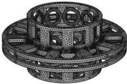
Figure 2 Model of the machine with finite element meshes
