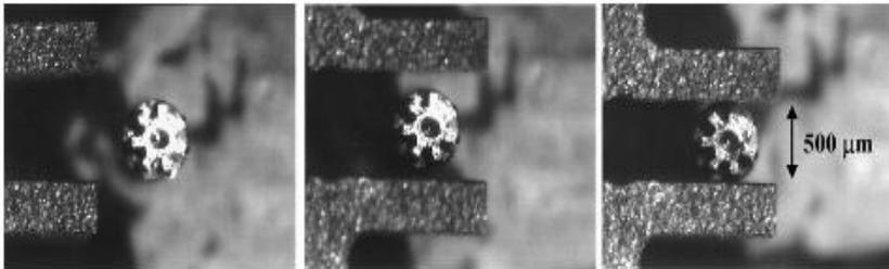
Fig. 12. Grasping action of the microgripper on the miniature gear.
