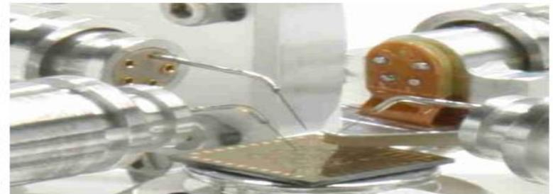
Figure 3 Microgripper end-effector interface
