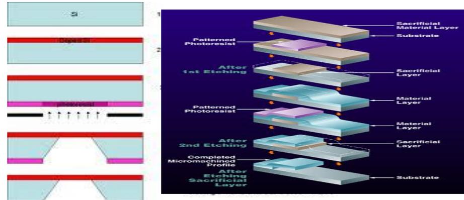
Bulk micromachining surface micromachining
