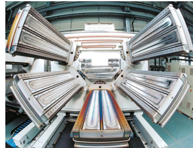
Target-configuration for metal strip coating (Von Ardenne)
