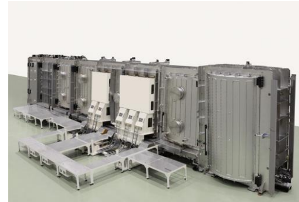
In-line sputtering system for display panel production (Ulvac)
