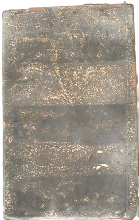
Lithium plating on graphite Anode
