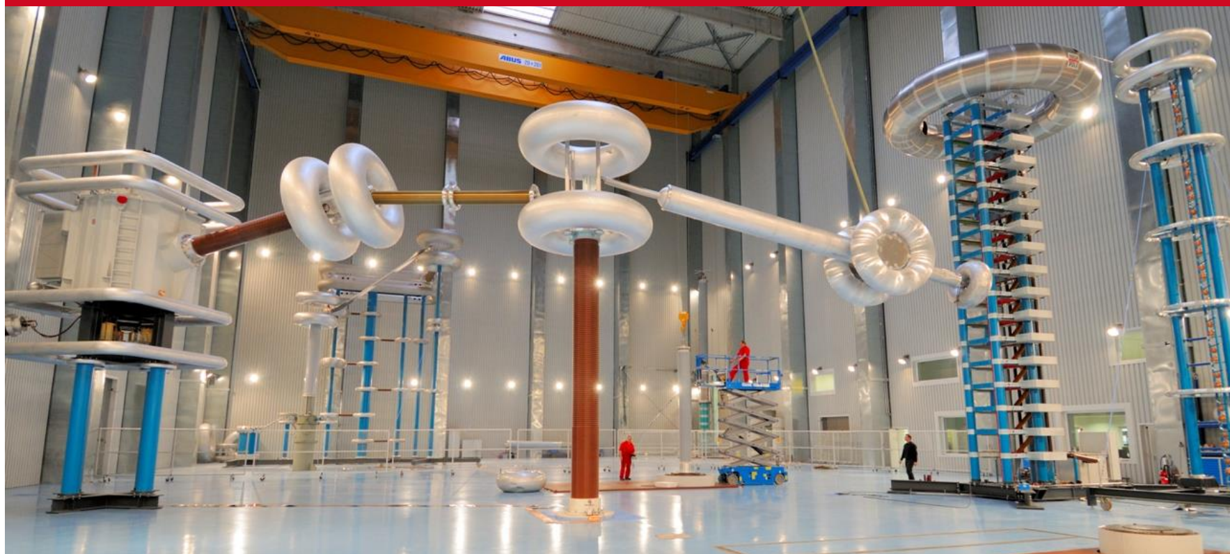
AC test system; 2400 kVA/1200 kV Courtesy of HSP, Germany
