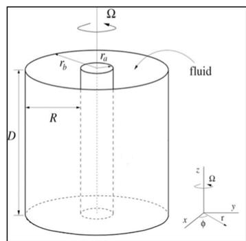
Figure 1. Rotating Concentric Cylinder.
