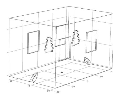
Ideal galvanic cell at an industrial scale for the Al electrodeposition on complex shaped cathodes.
