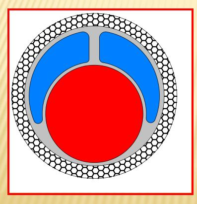
Blue – Coolant pathways (closed circuit) Red – Blood Grey- Teflon Mesh – Stainless steel-Pebax composite
