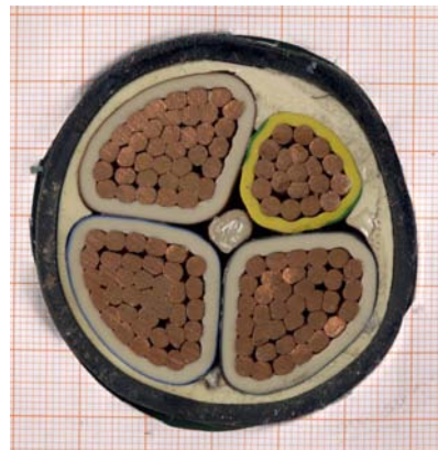
Figure 2: Low voltage segment cable
