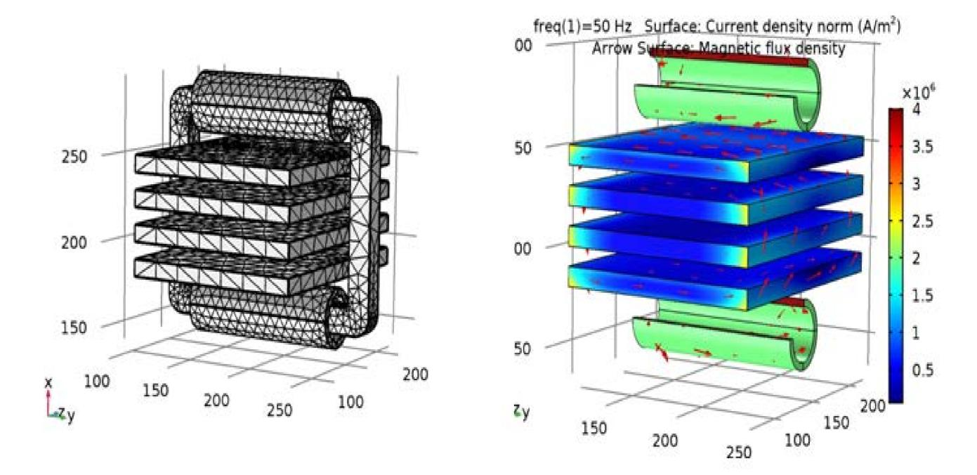
frequency based simulations are obtained using the COMSOL Multiphysics® AC/DC Module and the electric circuit of the primary bars is modeled separately [1]. The finite element (FE) simulation results are then compared to real time measurements.
