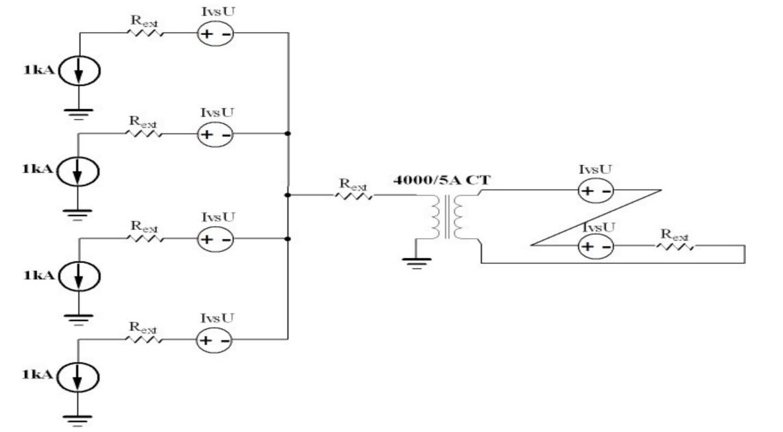
•Figure 2. Primary and secondary circuits coupled to the FE
