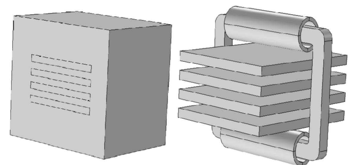
Figure 1. Geometry of the suggested model, a) enclosed by air, b) without air
