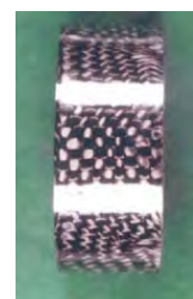
Resin impregnated YBCO pellets
