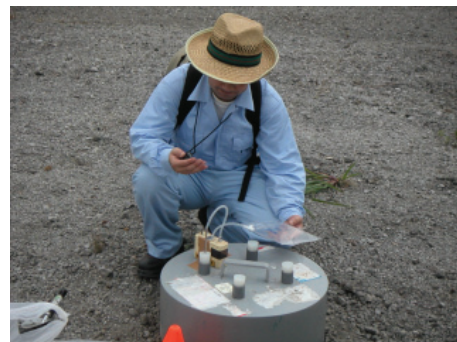
Figure 1. Static chamber method.
