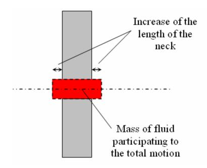
In modeling sound propagation through perforated sheets, losses are accounted by introducing corrections related to the distortion of flow and increment of the mass participating to the total motion of air
