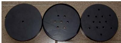
Five different resonators have been tested in 42 different configurations (in terms of perforation ratio, radius of the holes, thickness of the plate and air gaps).
