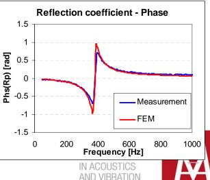
Once the acoustical formulation has been validated for modeling losses in plane perforated panels, it has been applied for predicting the sound transmission loss of reactive mufflers.
