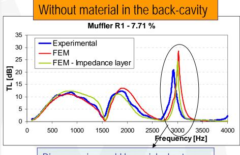
Discrepancies could be mainly due to small geometrical differences between real muffler and numerical model.
