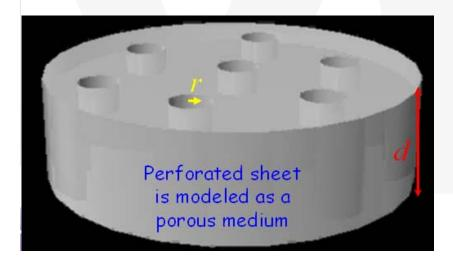
$$\sigma = \left(\frac{2 d}{r} + 4\right) \frac{\sqrt{2 \eta \omega \rho_0}}{2 \phi d}$$
