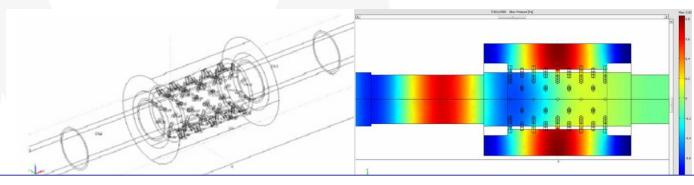
Mesh has been created according to the rule of 10 finite elements per wavelength.
