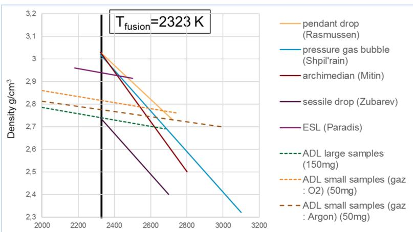
Figure 2. review of estimation of liquid alumina density[2,3] including ADL estimations with spherical approximation
