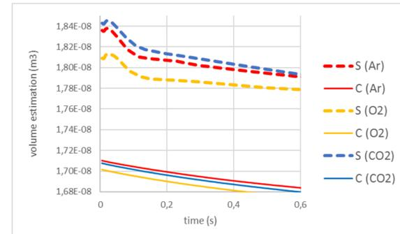
Figure 6 volume variation estimation after laser cut-off for various gas
