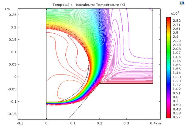
Figure 3. temperature map close to sample at rest
