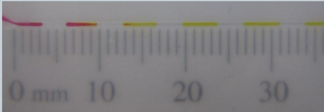
Demonstration of Two-Phase slug flow with chemical reaction
