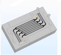
Face triangular mesh for the salt inlet surfaces.
