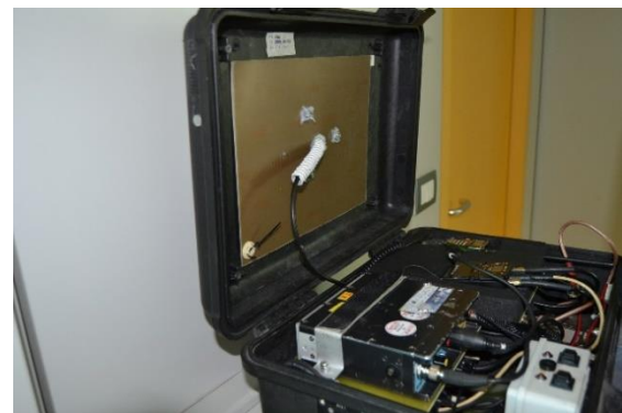
Figure 6. Antenna hosted in the top case of the motorcycle used for shooting events.
