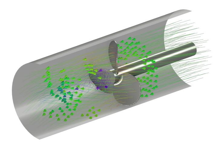
Figure 1 : Streamlines of flow resulting from propeller rotation
