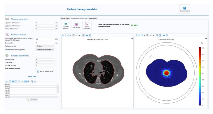
**Figure 1**: Simulation App overview for hadron therapy in COMSOL. Users set tumor and beam parameters to compute and visualize dose distribution on a segmented CT scan.
