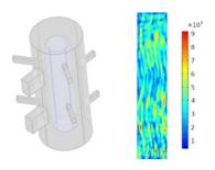
**Figure 1**: 3D geometry of the proposed MF microwave reactor, where the waveguides are easily identifiable. Right: cut plane showing the norm of the electric field generated in the reaction chamber. Colorbar values in V/m.
