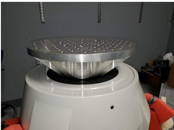
Shown here is the expander head that I bolted onto my electromagnetic shaker.
