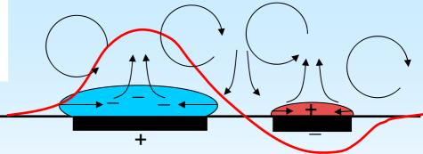
Distribution of electric potential along the electrodes (red line) induces tangential movement of the electric charge and thus eddies formation.
