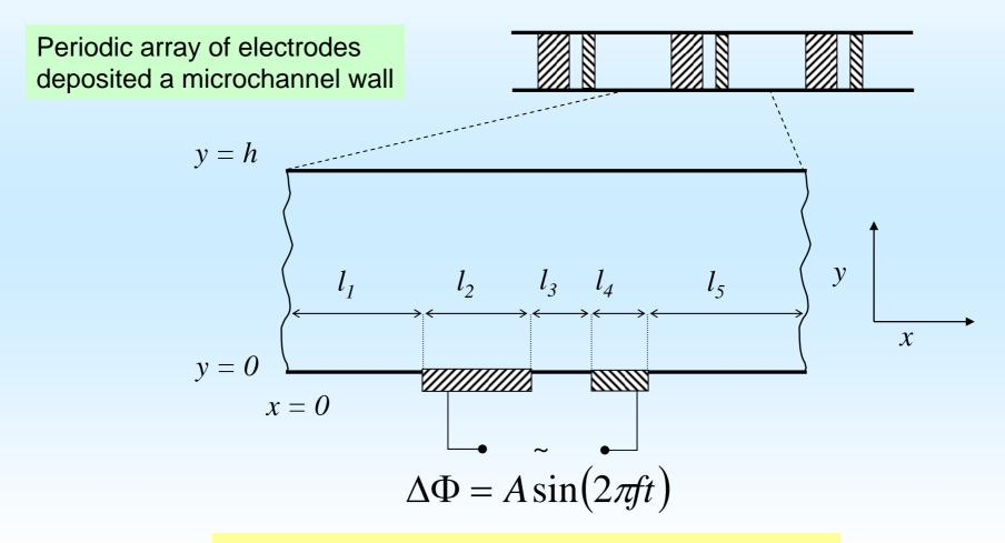
Geometry and dimensions of the microchannel ( $l_1 = l_5 = h = 10 \mu m$ ,  $l_2 = 5 \mu m$ ,  $l_3 = 2 \mu m$ ,  $l_4 = 3 \mu m$ ).
