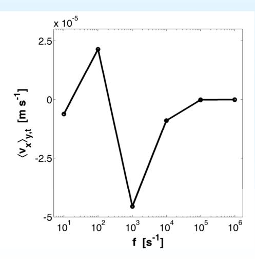
The dependence of the global velocity averaged over one period (1/f) on the applied frequency of AC electric field.
