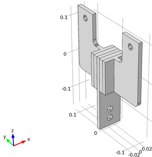
*Figure 1: Viscoelastic damping element.*
