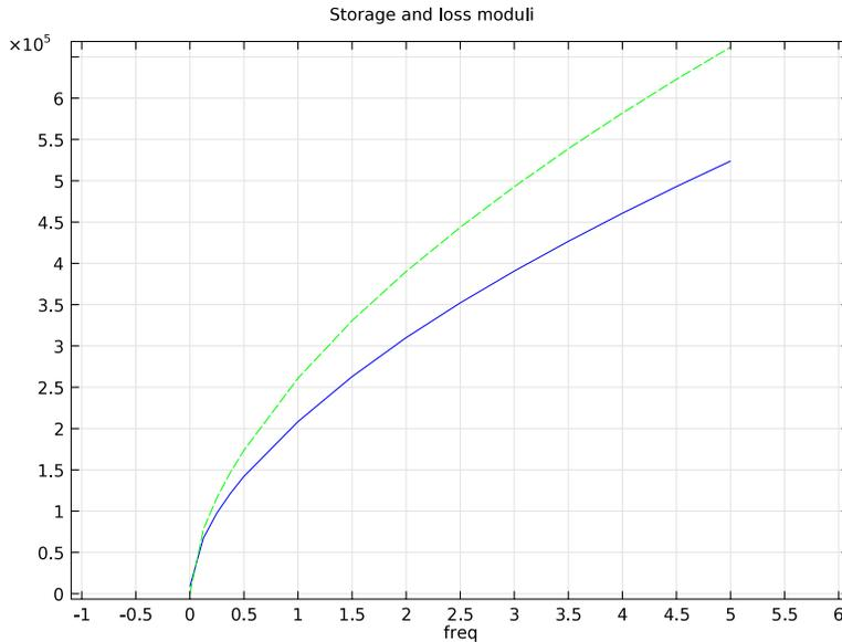
Figure 3: Viscoelastic storage modulus (solid line) and loss modulus (dashed line). Both quantities are normalized by 6.895 to simplify the comparison with Ref. 2.
