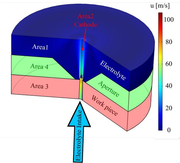
**Figure 2:** 3D sectional view of the velocity field of the non-isothermal electrolyte flow.
