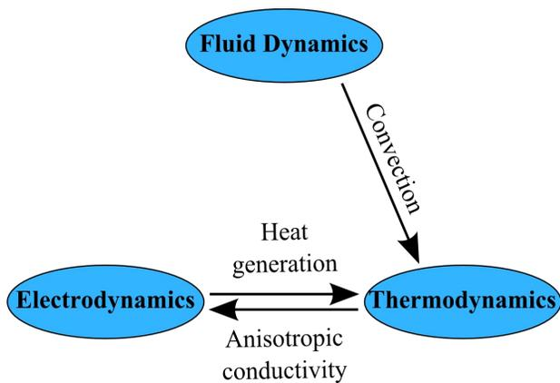
**Figure 1:** Applied physical phenomena and coupling.
