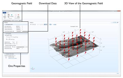
Use this tab to specify the geomagnetic field and the magnetic properties of the ore.
