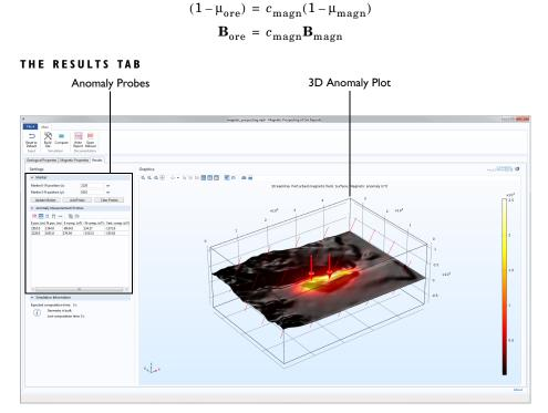
After the computation is complete, postprocessing occurs in the **Results** tab. On the right is presented a 3D plot of the anomaly of the geomagnetic field at the surface and the total (perturbed) field as streamlines.
