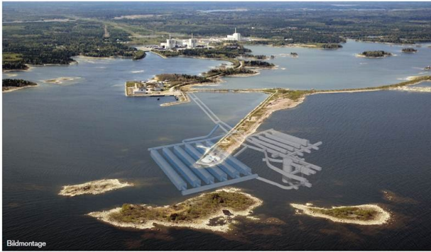
Figure 1: Illustration of the SFR Waste Repository vaults and tunnel system (SKB).
