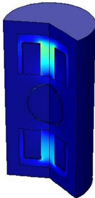
**Figure 1:** Magnetic flux density norm in MLS2EM.
