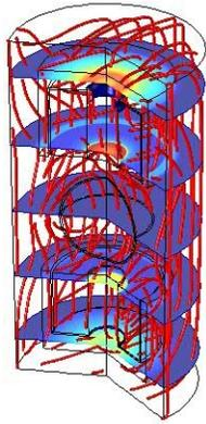
**Figure 2:** Visualization of magnetic flux density in MLS2EM.
