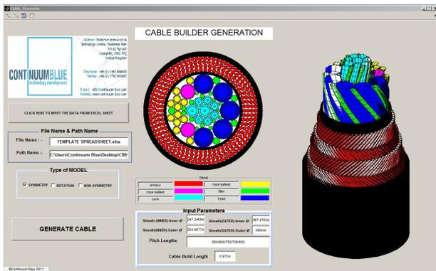
**Figure 2:** Screenshot of MATLAB® GUI developed to generate subsea cables in COMSOL using Livelink™ for MATLAB®.
