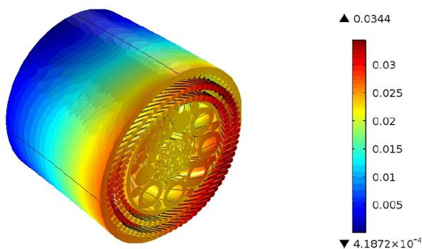
**Figure 1:** 3D cross-section of cable, illustrating cable displacement & slip conditions between armour wires & internal umbilical structures.
