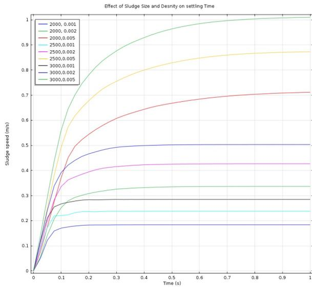
**Figure 1:** Plot on the effect of sludge density and size on the settling time.
