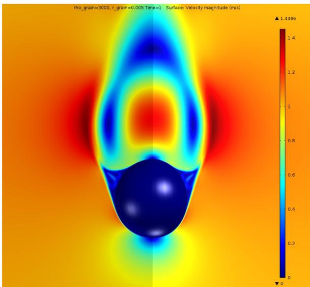
**Figure 2:** Typical velocity contour plots around the sludge
