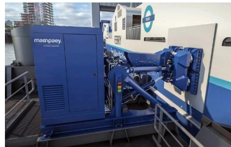
Figure 10. Magnetic mooring system: the magnets are located in the four black pads shown in the upper figure.
