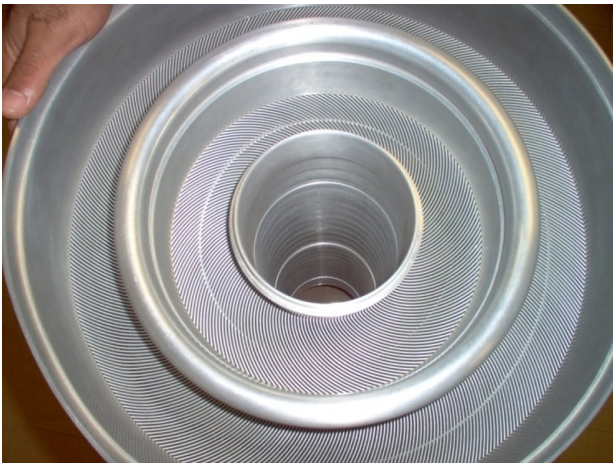
Figure 1: Top-down view of the HFIR core. The core's fuel plates are divided into an inner and outer elements, totaling 540 plates.
