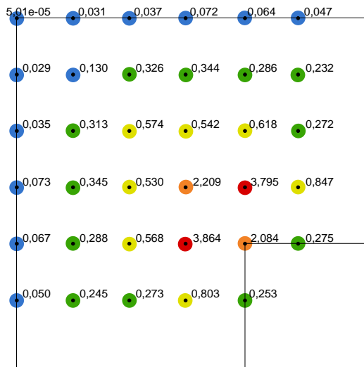
Figure 11 Percentage ratio of higher harmonic losses presented against a heat map of average point losses for the test grid. (Mean value of the three inner layers of test points shown).
