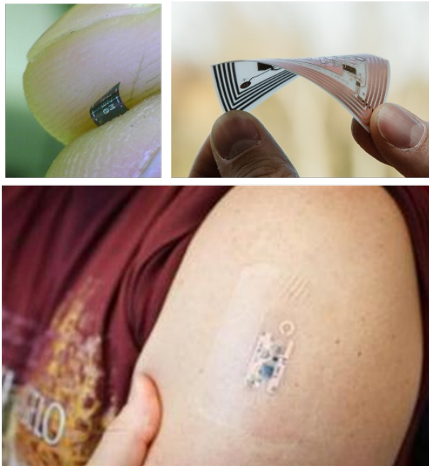
Figure 1: Ultra-thin chip bent between fingers (top left), Flexible monitoring tag (top right) and skin temperature sensor patch (bottom).
