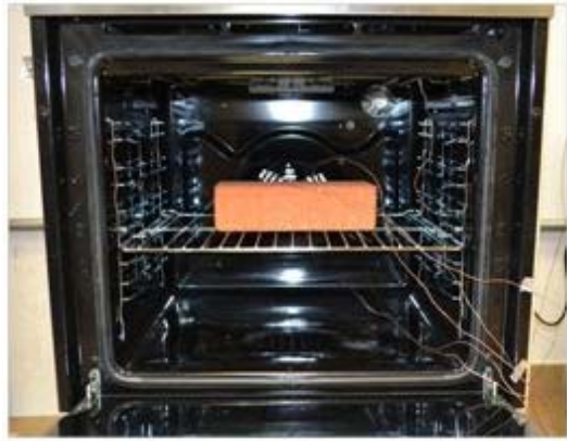
Figure 1. The oven and the position of the brick inside (Normative Oven Energy Class Test: EN 50304).
