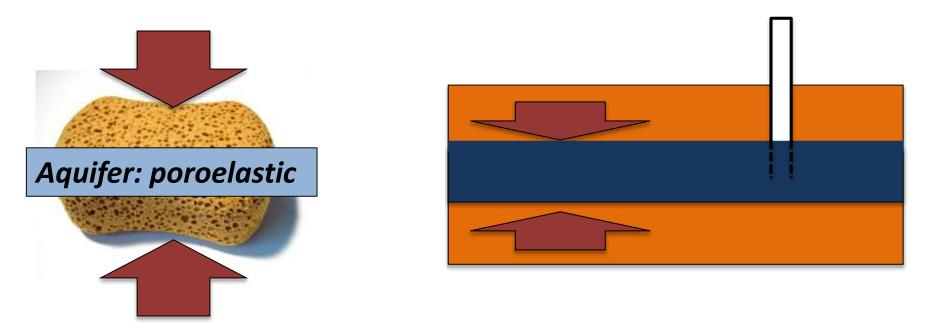
➤ Compression → decrease in pore space → Pore pressure/hydraulic head/water level rise
