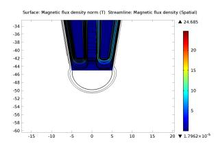
**Figure 2**: Magnetic field near the tip of the tool forming hemispherical field distribution (ball end).
