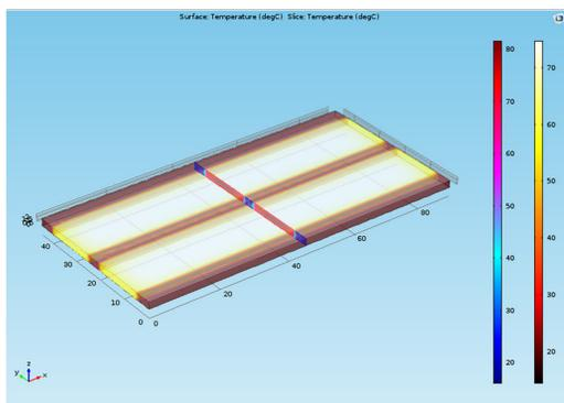
Figure 1. Whey gel pasteurization channels
