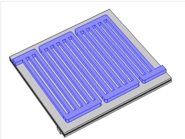
**Figure 1:** Description of DMFC flow field geometry
