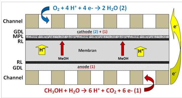
**Figure 2:** Function principle of a DMFC
