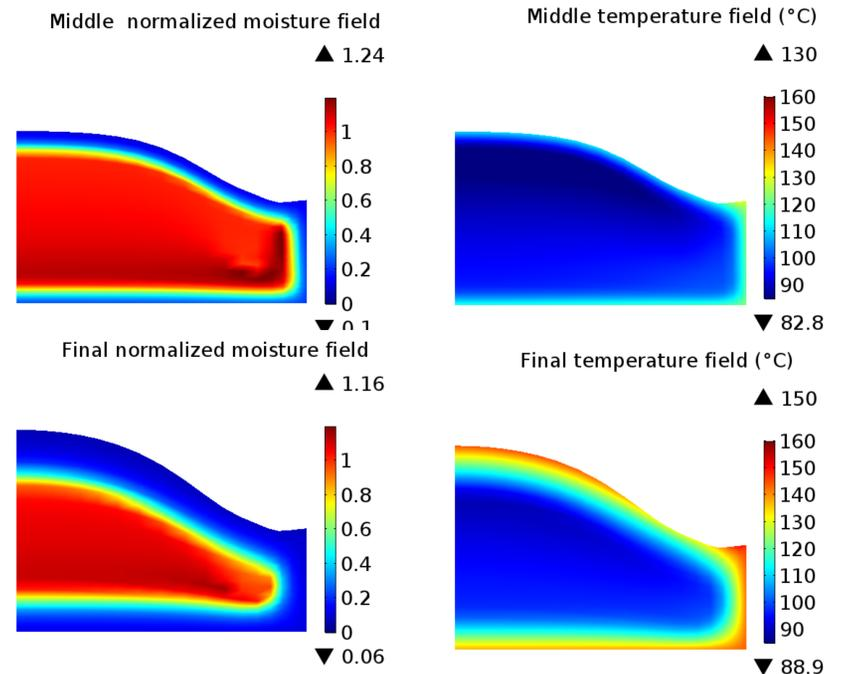
Temperature and normalized moisture fields at intermediate and final time
