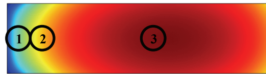
Figure 14. Textile moisture content profile after 1800 seconds
