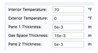
Figure 1: 1D Double Pane Gas Spaced Window Input Parameter Fields
