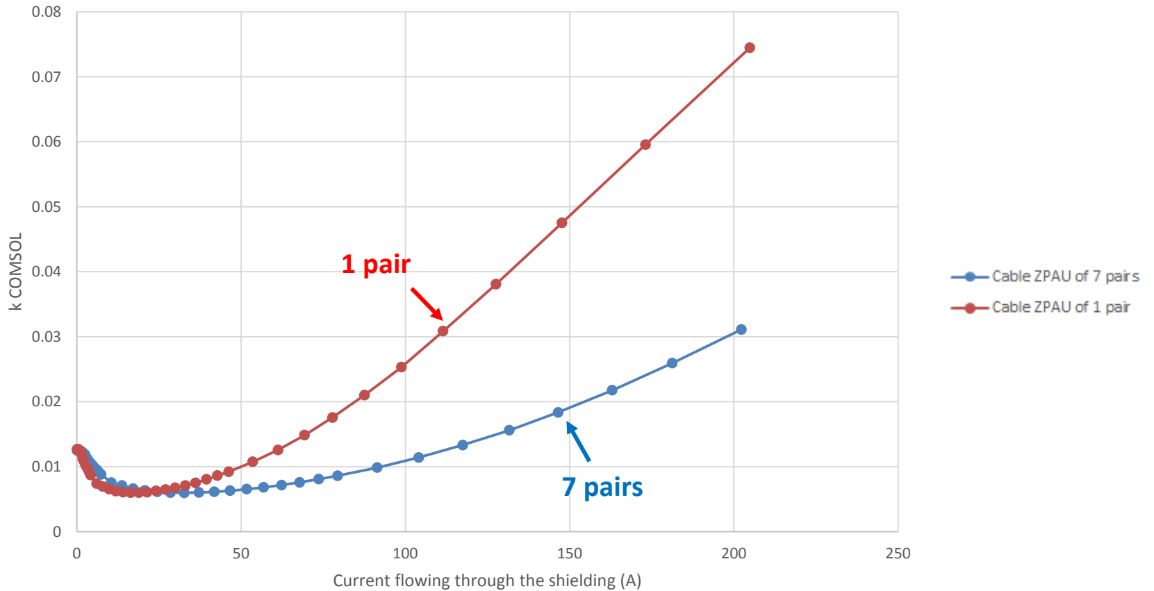
Reduction factor k from COMSOL Simulation for 50 Hz
