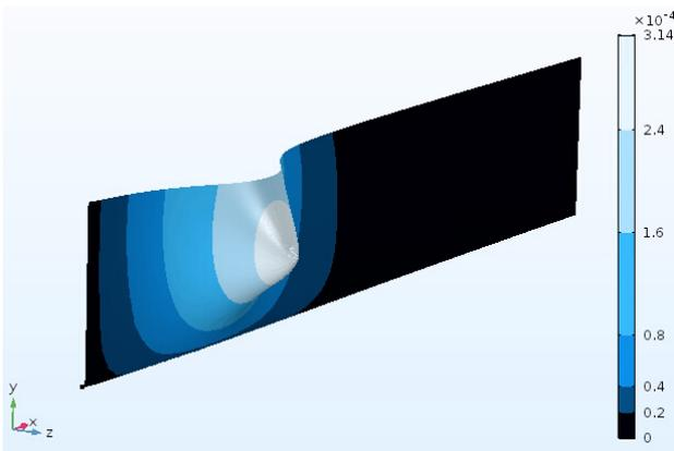
**Figure 1:** Representative Contour-Plot of the Space Charge Density [C/m<sup>3</sup>] emerging from an ionizing electrode for the Electrostatics part of the model.
