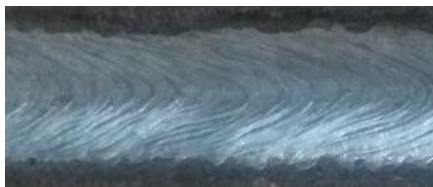
Representative films & bead on plate welds
