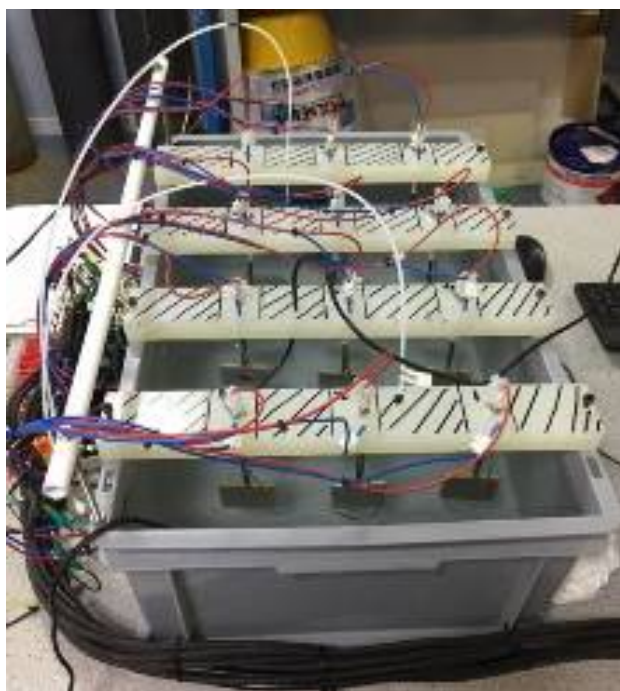
Figure 1: TSA coated corrosion sample coupons.
