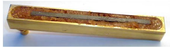
Figure 6. A manufactured sonar element mounted in a brass box.
